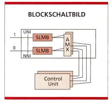
Bild 2. Blockschaltbild eines ATM Crossconnect ATM-CC-62. SLMB: Subscriber Line Module Broadband; TMB: Trunk Module Broadband; UNI: User Network Interface; ASN: ATM Switching Network; AMX: ATM-Multiplexer (ATM-Max); NNI: Network Node Interface.
