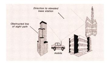
Fig. 2 The mechanism of radio propagation in urban areas
