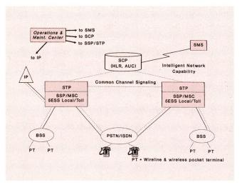
Fig. 5 Typical network architecture for personal communication
