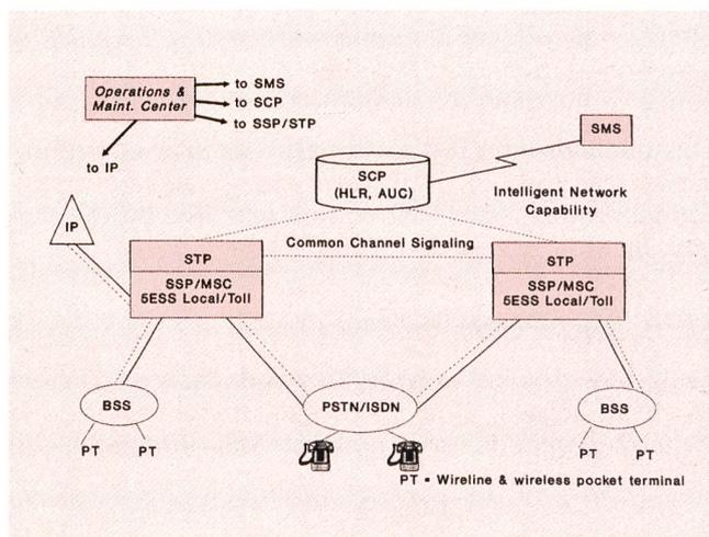
Fig. 5 Typical network architecture for personal communication
