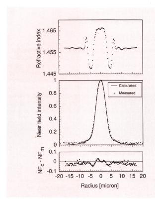
Fig. 5 Measured refractive index profile, the corresponding computed and measured near field, and their difference for a dispersion-flattened fiber
