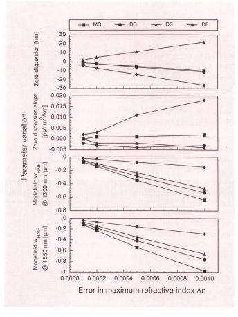
Fig. 2 Variation of optical transmission parameters versus error in maximum refractive index Δn
