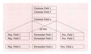
Fig. 6 The structure of the EDI notification
