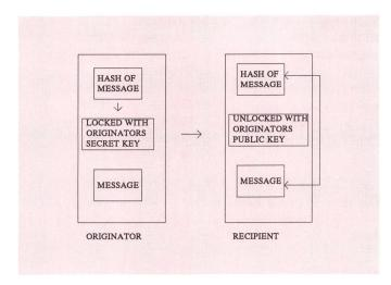
Fig. 4 Use of encryption for X.400 messages
