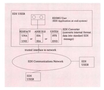
Fig. 1 Components of an EDI system
