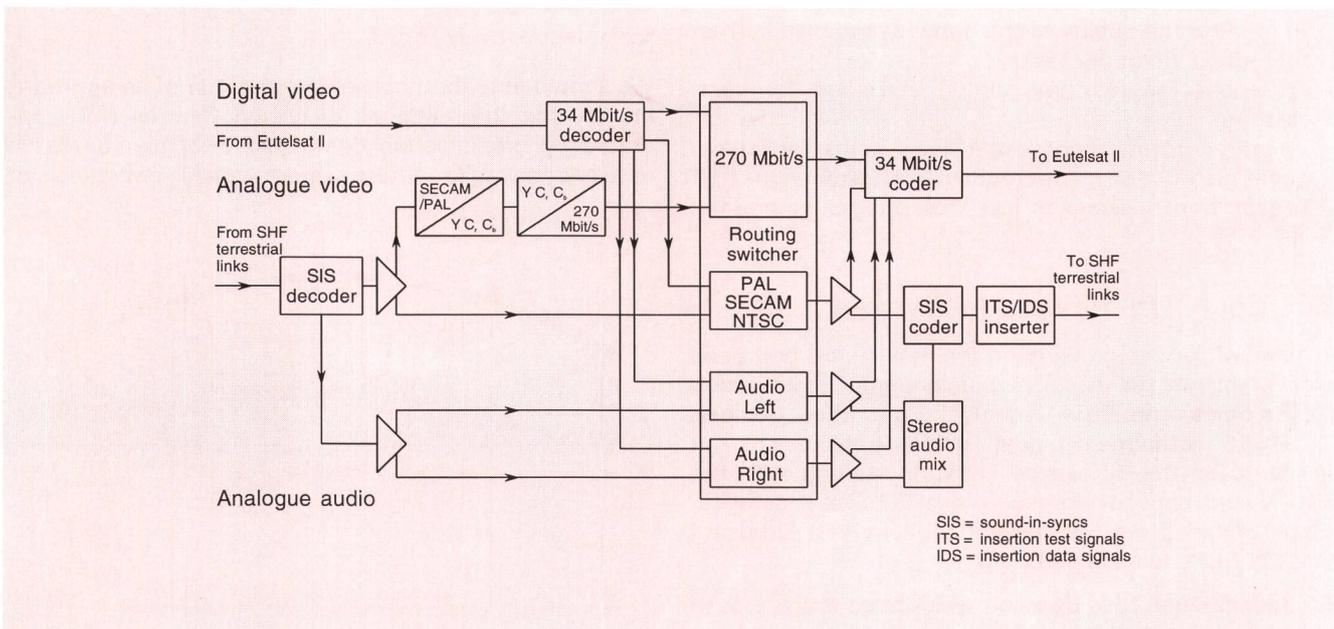
Fig. 3 Simplified schematic of video and audio configuration
