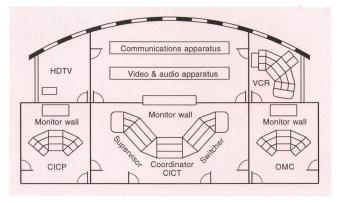
Fig. 1 Arrangement of operational areas
