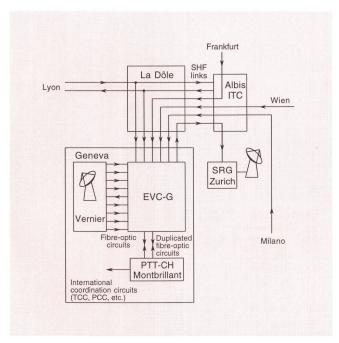
Fig. 5 Incorporation of the Eurovision Control Centre into the Eurovison network
