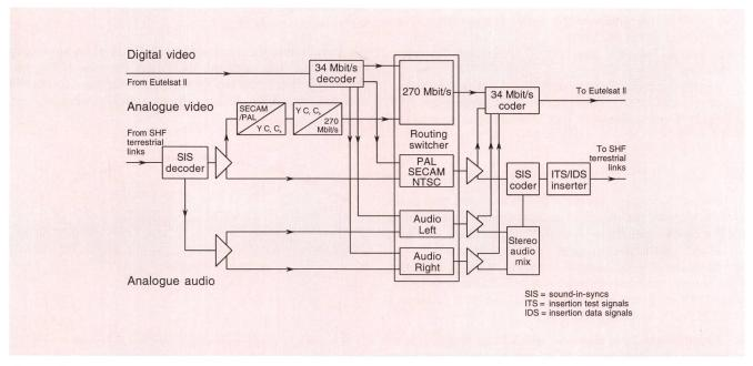
Fig. 3 Simplified schematic of video and audio configuration
