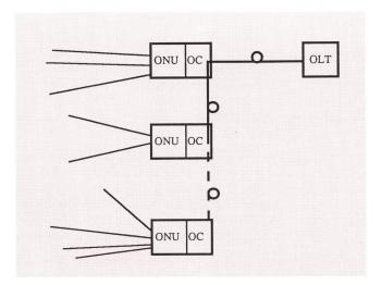
Fig. 7 Configuration PON bus/étoile
