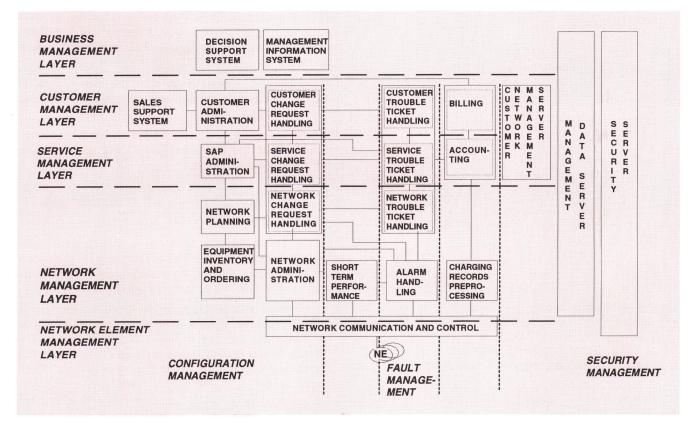
Fig. 14 NM/TI Ideal Architecture
