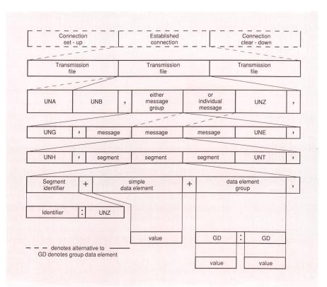
Fig. 4 Structure of an EDIFACT transfer file
