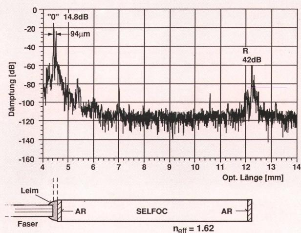
**Fig. 11 Transition fibre-Selfoc – Passaggio fibra-Selfoc**
