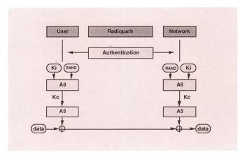
Fig. 2 Encryption of radio path
