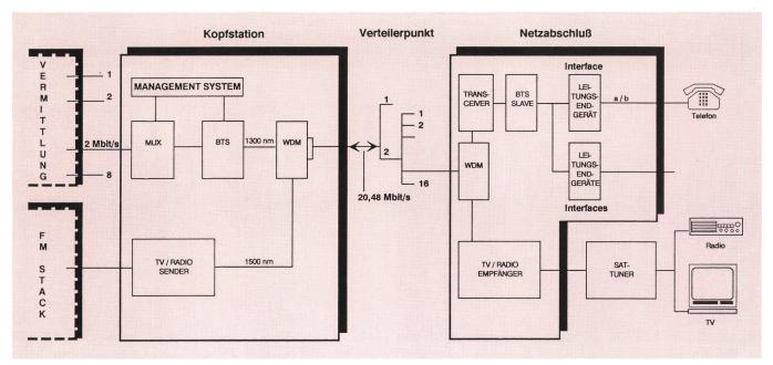
Passives optisches Netz Amsterdam BTS = Bit Transport System MUX = Multiplexer
