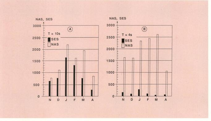
Fig. 8 Influence of the NAS definition on Severely Errored Seconds and on Non-Available Seconds performance.
