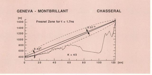
Fig. 2 Terrain elevation profile
