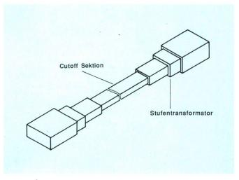
Fig. 6 Hochpass-Filter (Cut-off-Type)
