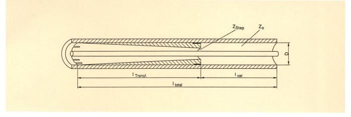
Fig. 6 Variable phase offset reflector element, overall length  $l_{total}\sim 500$  mm, adjustable length  $l_{var}=100$  mm Z-transformation length  $l_{\tau ransf}\sim 300$  mm Zo  $=50~\Omega$  (N-connectors)  $Z_{step}=33.3~\Omega$ , resulting reflection factor r=0.2 from 200 MHz to 18 GHz D =7.0 mm Ø
