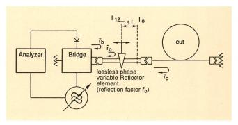
Fig. 2 Bridge, offset reflector set-up
