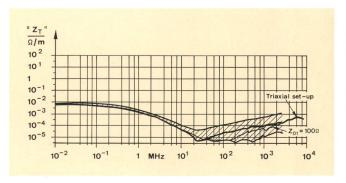
Fig. 12 Transfer impedance measurements for Sucoflex 104 cable. The envelope is the result of the measurements with the 50  $\Omega$  wire injection set-up taken at 120° apart around the circumference of cable. Before these measurements, this cable was used several months as a standard laboratory cable
