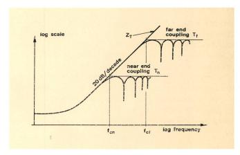
Fig. 3 Transfer impedance Z<sub>T</sub> and coupling transfer functions T<sub>n,f</sub> for a typical braided screen with negligible capacitive coupling Note:  $[Z_T] = \Omega/m$  and [T] = 1 have different dimensions The scales were chosen in that way that  $Z_T$  and T coincide for  $f < f_a$
