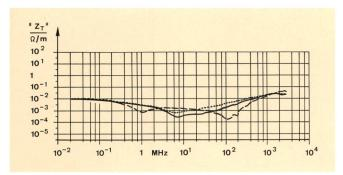
Fig. 14 RG 223/U measured at three different positions 120° apart around circumference of cable. 50  $\Omega$  wire injection set-up used
