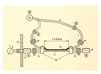
Fig. 5 polate inetallation for practical transfer impedance measurements
