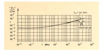
Fig. 10 Transfer impedance measurements for RG 58 C/U cable
