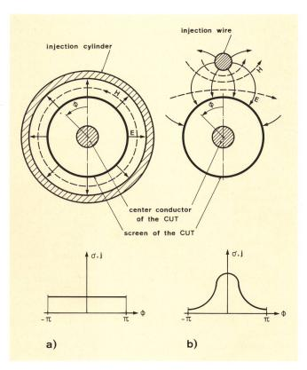
Fig. 1 Geometry and electric quantities in test set-ups
