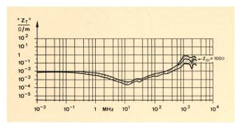
Fig. 13 Transfer impedance measurements for SA 07272 cable. The envelope is the result of three measurements with the 50  $\Omega$  wire injection set-up taken at 120° apart around the circumference of cable. Worst screening values found along the seam of foil screen
