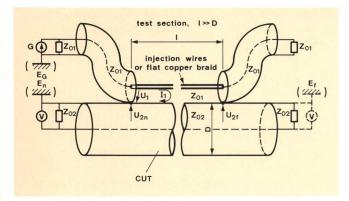
Fig. 4 New transmission type wire injection test set-up **Subscribts**
