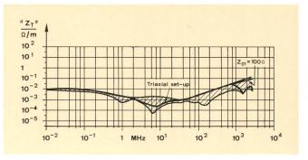
Fig. 11 Transfer impedance measurements for RG 223/U cable. The envelope is the result of the measurements with the 50  $\Omega$  wire injection set-up taken at 120° apart around the circumference of cable
