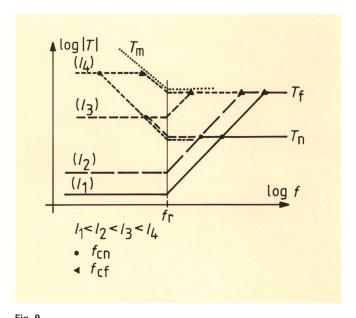
Effect of the cable length on coupling. Same cable as in Fig. 8 T(f) for different cable lengths. Only the envelope of the coupling is drawn.  $T_m$ : maximum attainable coupling  $(I \ge l_c)$ .
