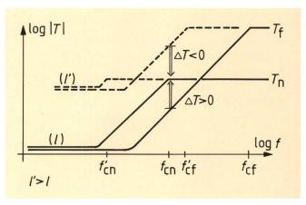
Fig. 11 Dependence of the couplings  $\mathcal{T}_n$  and  $\mathcal{T}_f$  on the length for a cable with following properties:
