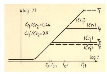
Fig. 10 Effect of the permittivity in the set-up on the coupling. Only the envelope is drawn. Reference cable: same parameters as in Fig. 8 Example:  $\epsilon'_{\rm rl}=0.9\cdot\epsilon_{\rm r2}\rightarrow\nu_{\rm rl}/\nu_{\rm r2}=1.05\rightarrow f'_{\rm cf}=6.7\cdot f_{\rm cf},$  for  $f\!>\!f'_{\rm cf}$ : Env  $(T')/{\rm Env}$  (T)=6.7=16 dB.
