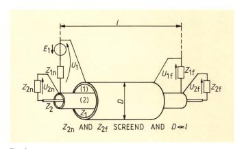
Concept of the tricoaxial test set-up
