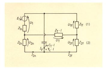
Fig. 5 Equivalent circuit of the set-up for low frequencies, i.e. for an electrically short cable  $(I \! \ll \! \lambda)$ , with general load conditions
