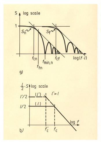
Fig. 7 a) The summing function S(lf) for near and far end couplings b) The envelope of the product (l/2) S as function of frequency, with l as parameter.  $f_{\rm C}$ : cut-off frequency
