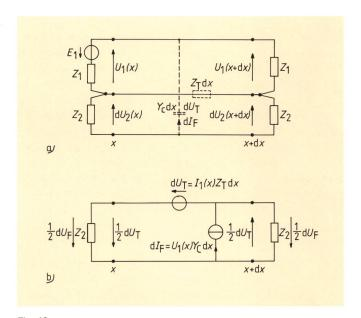
Fig. 16 Coupling of an elementary short section dx, a) total circuit, b) circuit (2).
