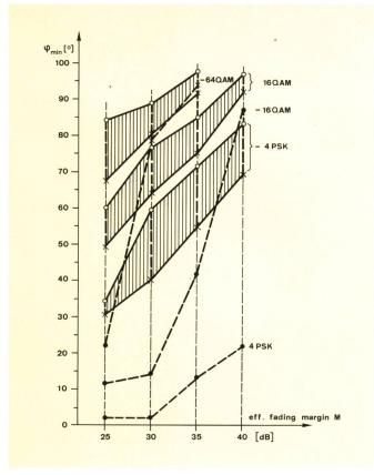
Antenna: 7 GHz, 3 m Ø, Gain: 45 dB Minimum angular separation (for two interferers)
