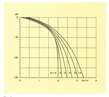
Fig. 4 Adjacent-channel suppression at the regenerator (ideal Nyquist-filtering, 50 %/50 %)
