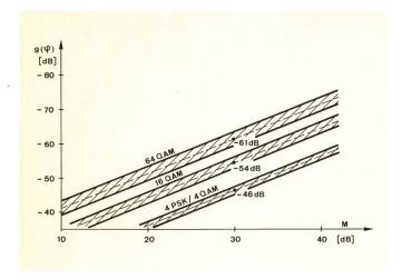
Fig. 5 Minimal relative antenna discrimination g  $(\phi)$  in function of eff. fading margin M
