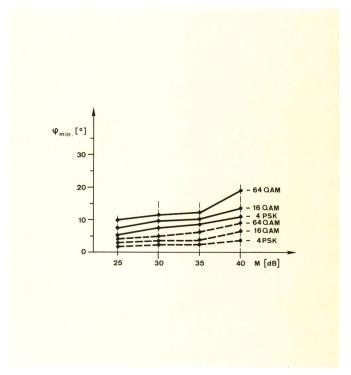
Antenna: 11 GHz, 3 m Ø, Gain: 48 dB (offset-type) Minimum angular separation (two interferers) maximum for all combinations of polarizations
