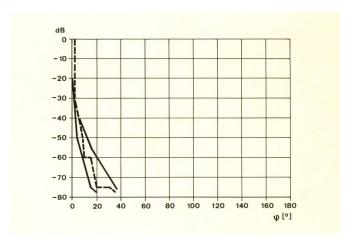
Fig. 8 Radiation pattern, Antenna 11 GHz, 3 m Ø (offset-type)
