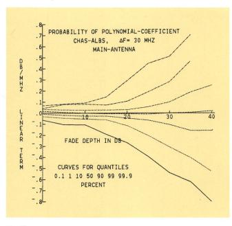
Fig. 10 Probability of the amplitude slope dispersion, main-antenna
