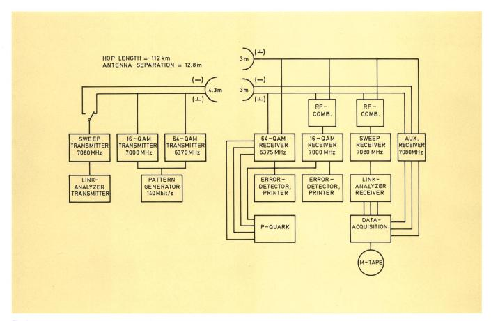
Fig. 1 Test configuration
