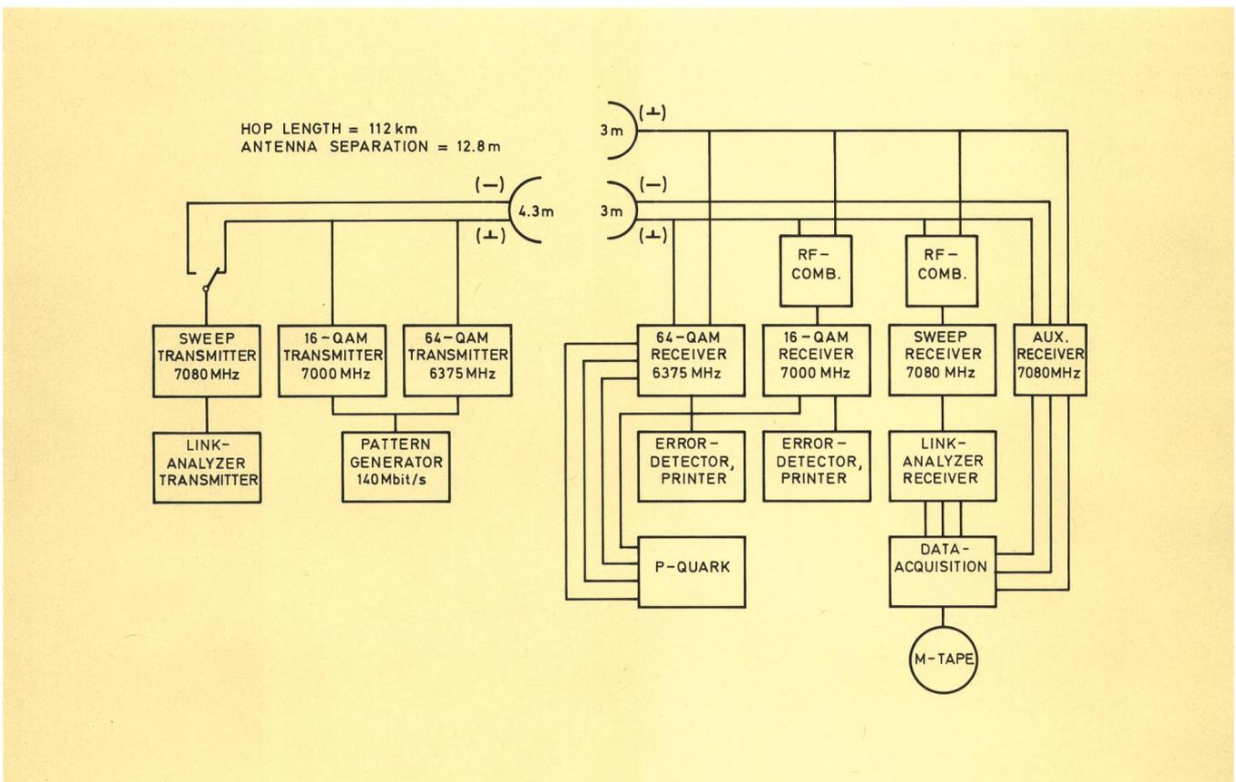
Fig. 1 Test configuration
