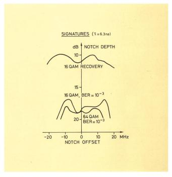
Fig. 2 Signatures of the digital radios
