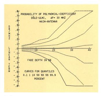
Fig. 20 Probability of the amplitude slope dispersion, main-antenna
