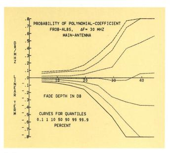
Fig. 16 Probability of the amplitude slope dispersion, main-antenna
