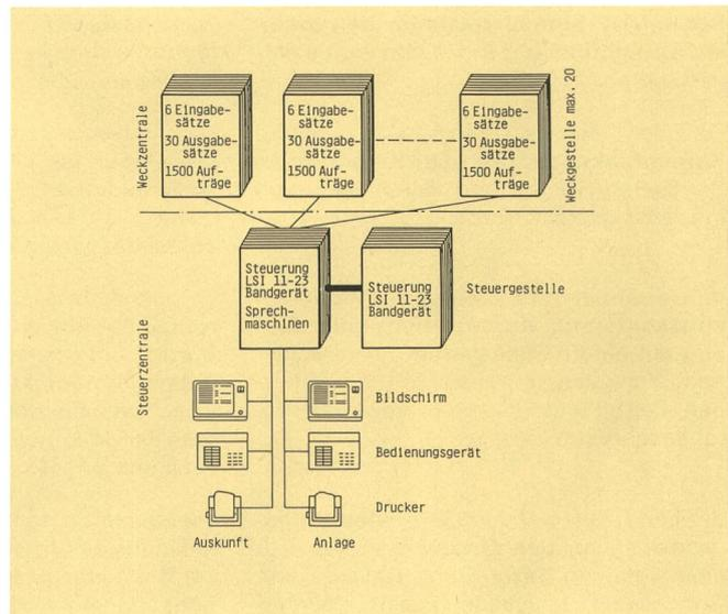
Fig. 1 Configuration of the wake-up call system, WA 490
