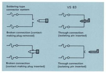
Isolating terminal block, basic diagram
