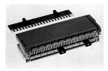
Fig. 15 Printed circuit multiple
