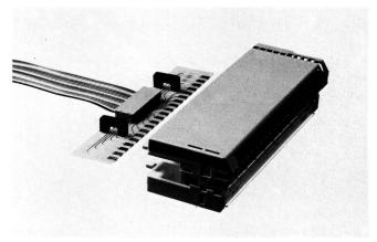
Fig. 14 Connection of ribbon cable
