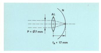
Fig. 2 Optical equivalent of the human eye AL Eye lens
