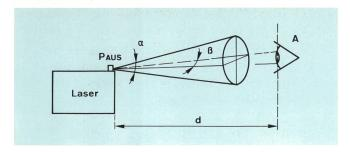
Fig. 5 Light exit from laser diode
