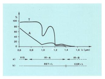
Fig. 3 Transmission and absorption in the eye
