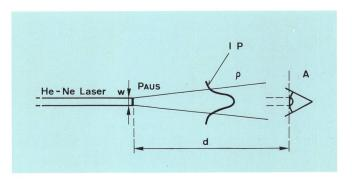
Fig. 10 Light exit from a He-Ne-laser
