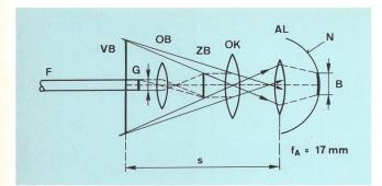
Fig. 6 Principle of imaging by a microscope
