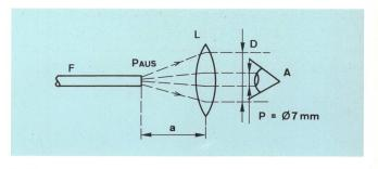
Fig. 8 Single lens magnifying glass – light exit from fiber F Fiber A Eye  $P_{AUS}$  Radiant power P Pup
