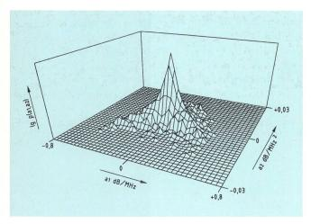
Fig. 5 Probability density function of the coefficients of the fit-polynomial attenuation A(f) =  $a_0 + a_1 f + a_2 f^2$ , (1 259 348 sweeps),  $-15 \, dBm > a_0 > -85 \, dBm$  Main antenna, vertical, in-line signal
