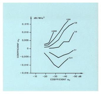
Fig. 11 Quantiles of the distribution of the parabolic term  $a_2$  Main antenna, horizontal, in-line
