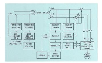
Fig. 1 Block diagramm of the field experiment
