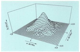
Fig. 6 Probability density function of the coefficients of the fit-polynomial attenuation  $A(f)=a_0+a_1f+a_2f^2$ , (1 124 645 sweeps),  $-45\,dBm$  Main antenna, vertical, cross-polar signal
