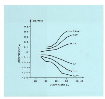
Fig. 9 Quantiles of the distribution of the linear term a<sub>1</sub> Main antenna, vertical, cross-polar
