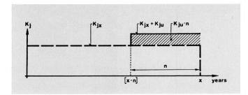
Fig. 7 Calculation of costs of invested capital  $(K_j)$  for upgrading of an electromechanical system
