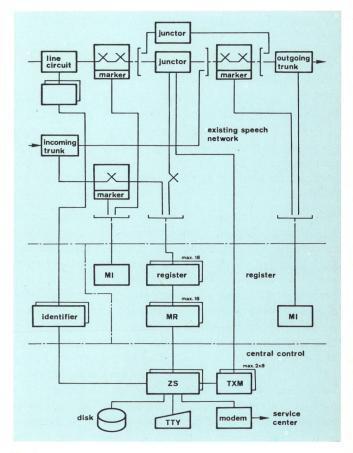
Fig. 5 Blockdiagram modernisation of crossbar exchanges
