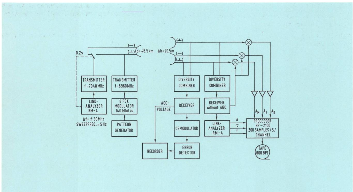
Fig. 1 Block diagram of the field experiment
