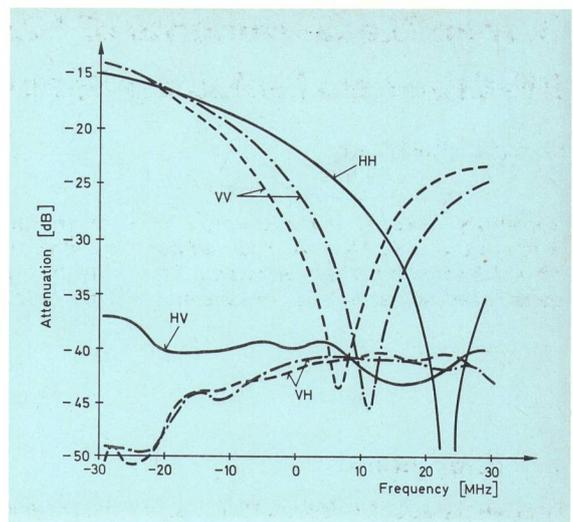
$A_D(f)$  Amplitude frequency-response of the diversity-antenna signal (vertically polarized reception)
