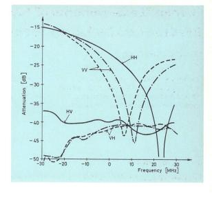
$A_D(f)$  Amplitude frequency-response of the diversity-antenna signal (vertically polarized reception)
