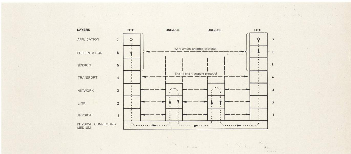
Fig. 5 Layer structure ISO/OSI (International Standards Organisation/Open System Interconnection), for CCITT data network of Fig. 3
