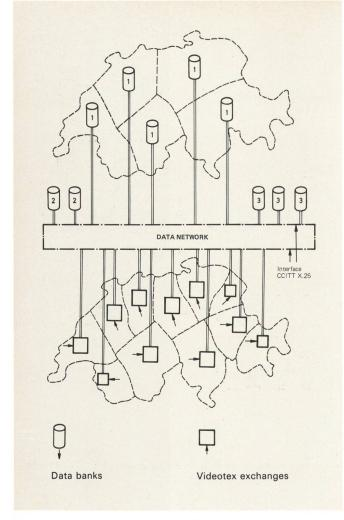
Fig. 11 Long range solution for the realization of the Videotex service
