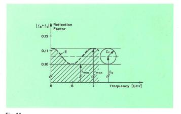
Extraction of  $\underline{r}_c$  (ripple E) by dividing the difference  $r_{max} - r_{min}$  by two.  $\underline{r}_c$  is the reflection factor of the connector under test (including the reflection of the standard connector at C of Fig. 10)
