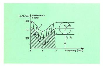
Fig. 13 Detail A, converted to reflection factor. Elimination of  $r_d$  by averaging out F. Ordinate values of shaded area corresponds to the sum  $|\underline{r}_b + \underline{r}_c|$
