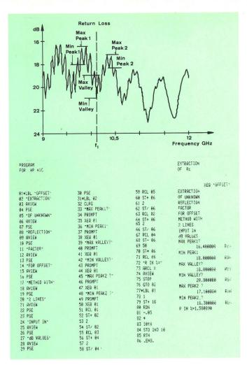
Fig. 15 Extraction of  $\underline{r}_{c}$  at  $f_{1}$  with programmable pocket calculator
