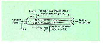
Fig. 9 Impedance step line reflection (with  $\epsilon_r \!=\! 1.5)\, r_{offset} \sim \! 20$  dB return loss
