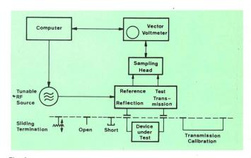
Fig. 4 Automatic network analyzer block diagram
