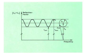
Fig. 7 Summation of reflection phasors according to set-up of Figure 6
