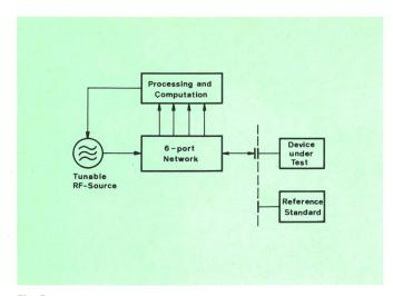
Fig. 5 Six-port measuring configuration
