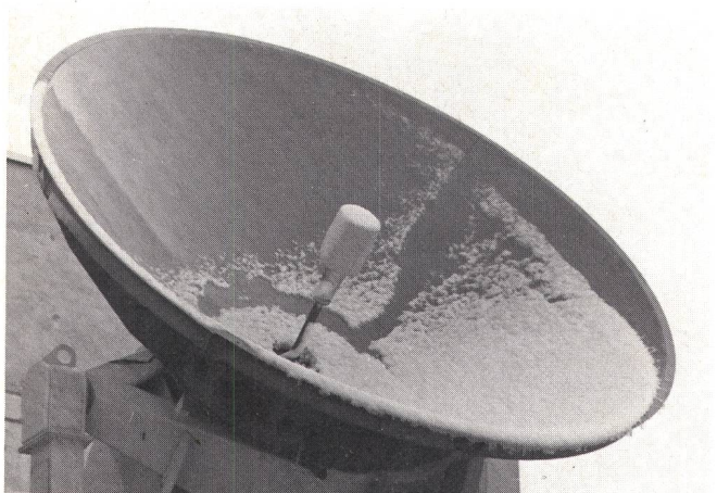
Fig. 8 Melting snow on the receiving antenna on 3 April 1979 at 07.40 hours
