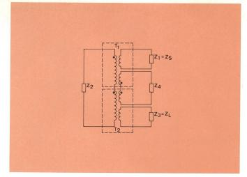
Fig. 4 Hybrid circuit with transformers
