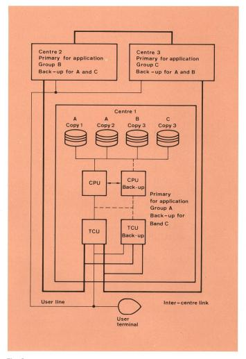
Fig. 3 Configuration of the computer network for the TERCO system Centre internal or centre external switching of operations to back-up:  $<\!30~\text{s}$
