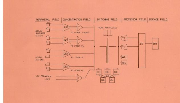
Fig. 1 IFS Network Structure of one Plane AKT Analog concentrator
