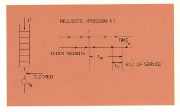
Fig. 15 Model 1 for Calculation
