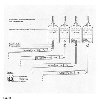
Corrosion experiment with calcium solutions of different pH values
