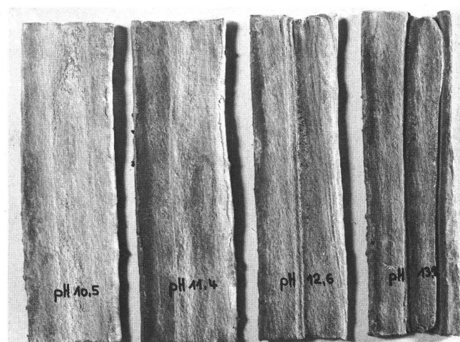
Fig. 12 Condition of the pure lead samples after termination of the experiment
