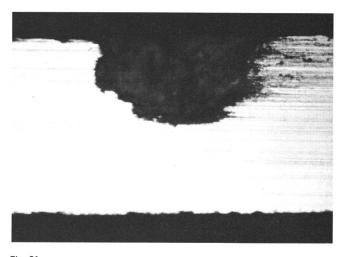
Cross-section through a crater-shaped corrosion in the lead sample illustrated in Figure 19 (magnification 20-fold)
