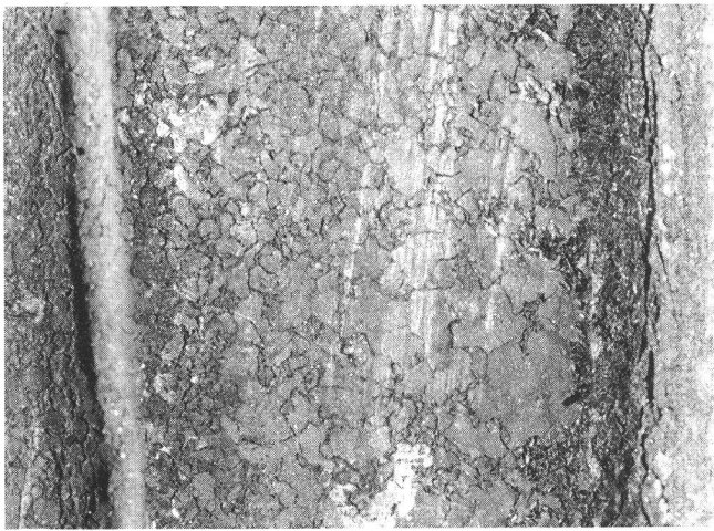
Fig. 14 There are no corrosion products on the surfaces rinsed with strongly basic solutions, indeed they have been strongly etched As a result the grain boundaries are clearly visible in this enlarged section of the sample treated at pH 13.1 (magnification 5.1-fold)
