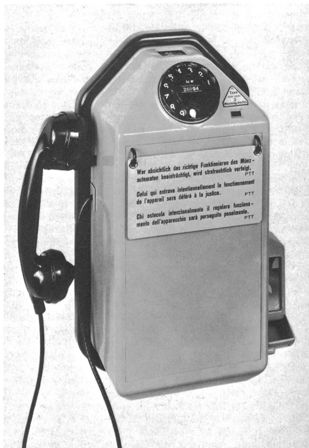
Fig. 1 The M-type coinbox telephone in the form in which it is still encountered – in service since 1948
