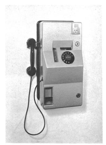
Fig. 3 The AZ 1 coinbox telephone, in service since 1966
