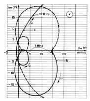
Fig. 13 Results of the input and output admittance measurements: curve a) is the plot of  $Y_{\rm in}$  curve b) is that of  $Y_{\rm out}$
