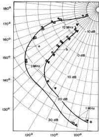
Fig. 11 Loop-gain measurement results Results with the 'classical method': curve a) for  $R_v=18\,\Omega$
