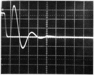
Fig. 12a+b Responses of test-amplifier to step input Time scale = 0,1  $\mu$ s/div. a)  $R_{\nu}=$  18  $\Omega$  b)  $R_{\nu}=$  43  $\Omega$
