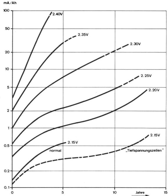
Fig. 3 Time-behaviour of currents as a function of voltage
