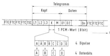
Fig. 8 Telegram format in the peripheral telegram system
