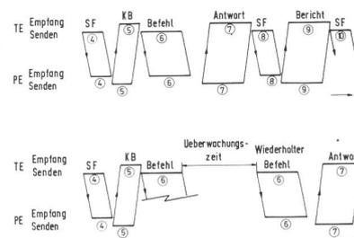
Fig. 7 Compelled telegram exchange, normal and interrupted
