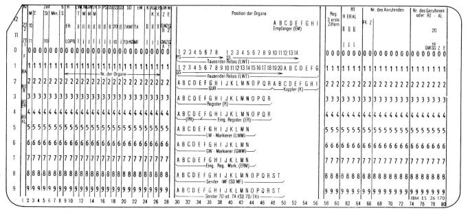
Front for manual check of fault print-out
