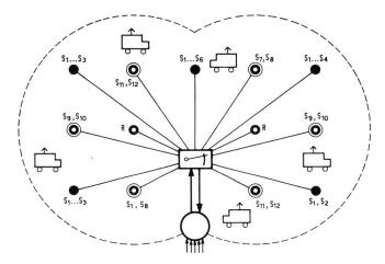
Fig. 1 Principle of the structure of a mobile radio-telephone network comprising a calling (or control) channel R and 12 speech channels  $S_1...S_{12}$  (the numbers assigned to the channels are chosen at random)
