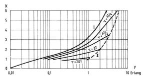
Fig. 7 Tolerable traffic y when one demands 95% assurance of finding a free channel from x channels available for use ( $\triangle T$ : average occupation time;  $\triangle \tau$ : average waiting time)
