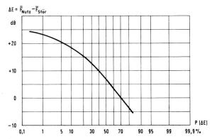
Fig. 8 Probability of channel commutation P ( $\triangle$ E) in a 1 km long street section in relation to the average HF S/N ratio
