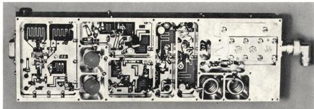
Quarzstabiler 4 GHz-Oszillator
