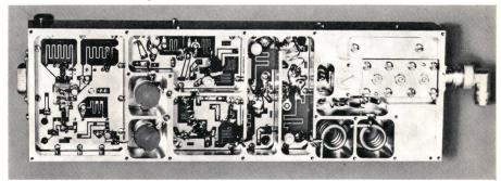
Quarzstabiler 4 GHz-Oszillator
