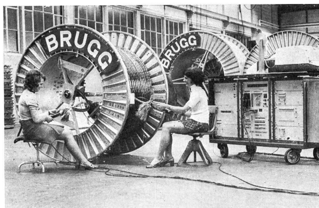
Fig. 4 Operators testing a factory length of cable by means of automatic tester KMA-3b
