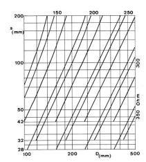
Fig. 8  $s = F \ (D, \, Z_o, \, d) \ mit$   $Z_o = 150...350 \ \Omega$   $d = 28, \, 32, \, 42 \ mm \ Hohlseil$
