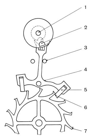
Fig. 2. Ankergang – Ancre
