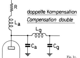
$$R = \frac{\Omega_3}{\omega_3 C} = \frac{279\,000}{\left[\frac{f_3}{\text{Me/s}}\right] \cdot \left[\frac{C}{\text{pF}}\right]} \quad \text{(ohms)}$$
