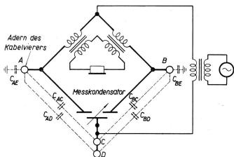
$k_2 = 0$  wenn  $C_{AC} + C_{AD} + \frac{1}{2}C_{AE} = C_{BC} + C_{BD} + \frac{1}{2}C_{BE}$
