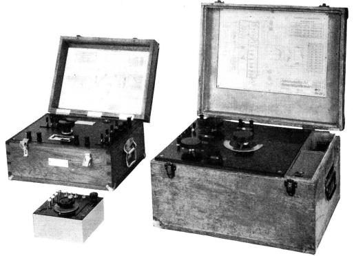
${\bf Fig.~8} \\ {\bf Kapazit\"{a}ts\text{-}Unsymmetrie-} \\ {\bf Messbr\"{u}cke} \\$
