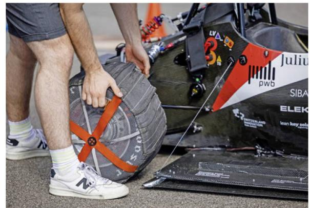
ABOVE: Putting on warm tyres. The suction device is visible close to the ground.
