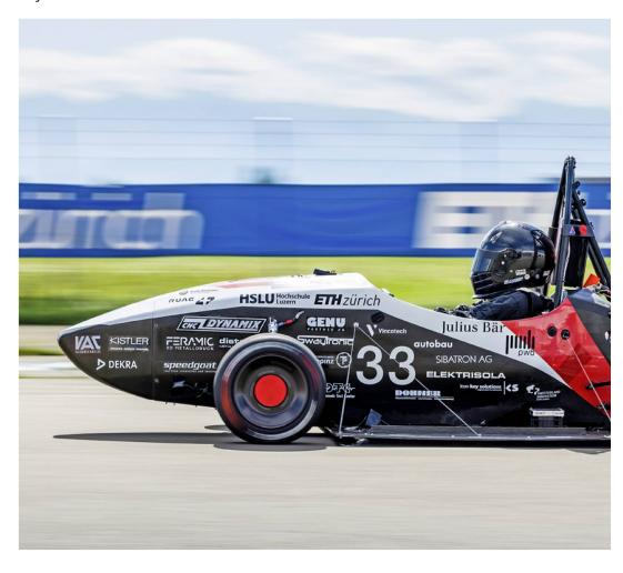
What a strange sight. Zip away, then brake. Like breathing in and out just once. Barely three seconds elapsed before the electric car and its driver Kate Maggetti came to a halt again. The vehicle needed just 0.956 seconds and a distance of a little over ten metres to reach a speed of 100 km/h.
