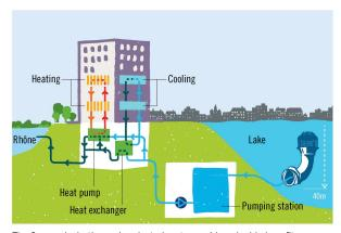
The Geneva hydrothermal project aims to provide a double benefit. In winter, energy is taken from the water by means of a heat pump in order to heat a building. In summer, a building can be cooled using cool water taken from the depths.
