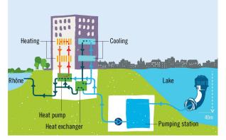
The Geneva hydrothermal project aims to provide a double benefit. In winter, energy is taken from the water by means of a heat pump in order to heat a building. In summer, a building can be cooled using cool water taken from the depths.
