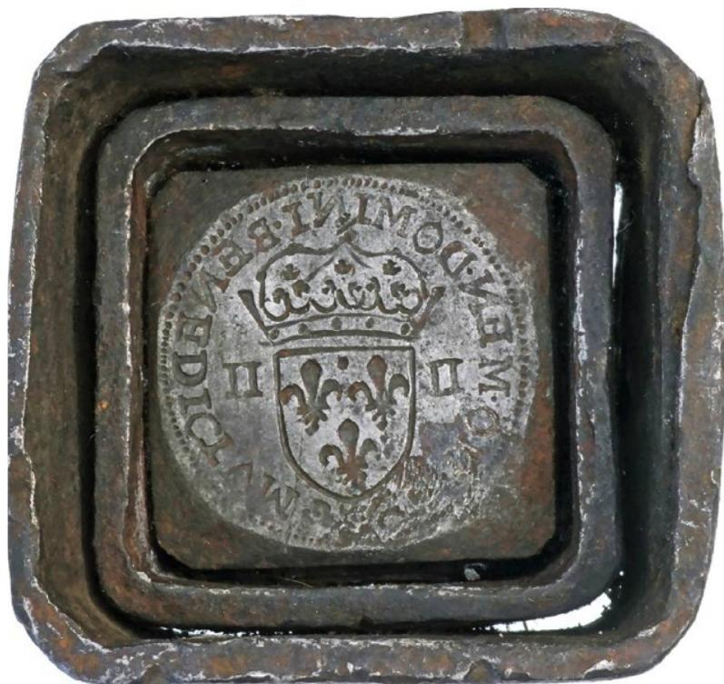
A moveable iron die for the falling-hammer or screw-press striking of the quarter ecu coin.
