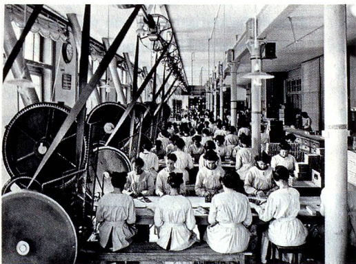
Kempthal 1896: Assembly line work in the Maggi factory. Mechanical transmission equipment powered the packing conveyor before electrification
