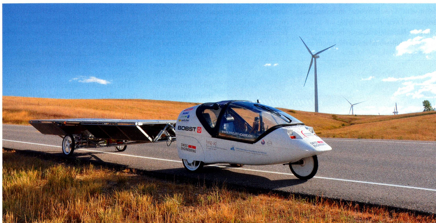
The "Icurette", a converted Twike, is powered by solar and wind energy
