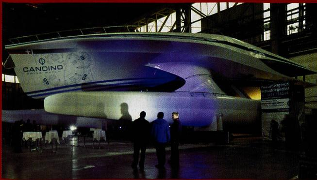
It's taken just 13 months to build, but now one of the most remarkable Swiss inventions in the field of transport is almost ready for its historic launch. Called PlanetSolar, this sleek, 32 metre long catamaran is powered only by sunlight. If its sea trials are a success, it could pave the way for a completely new generation of shipping.
